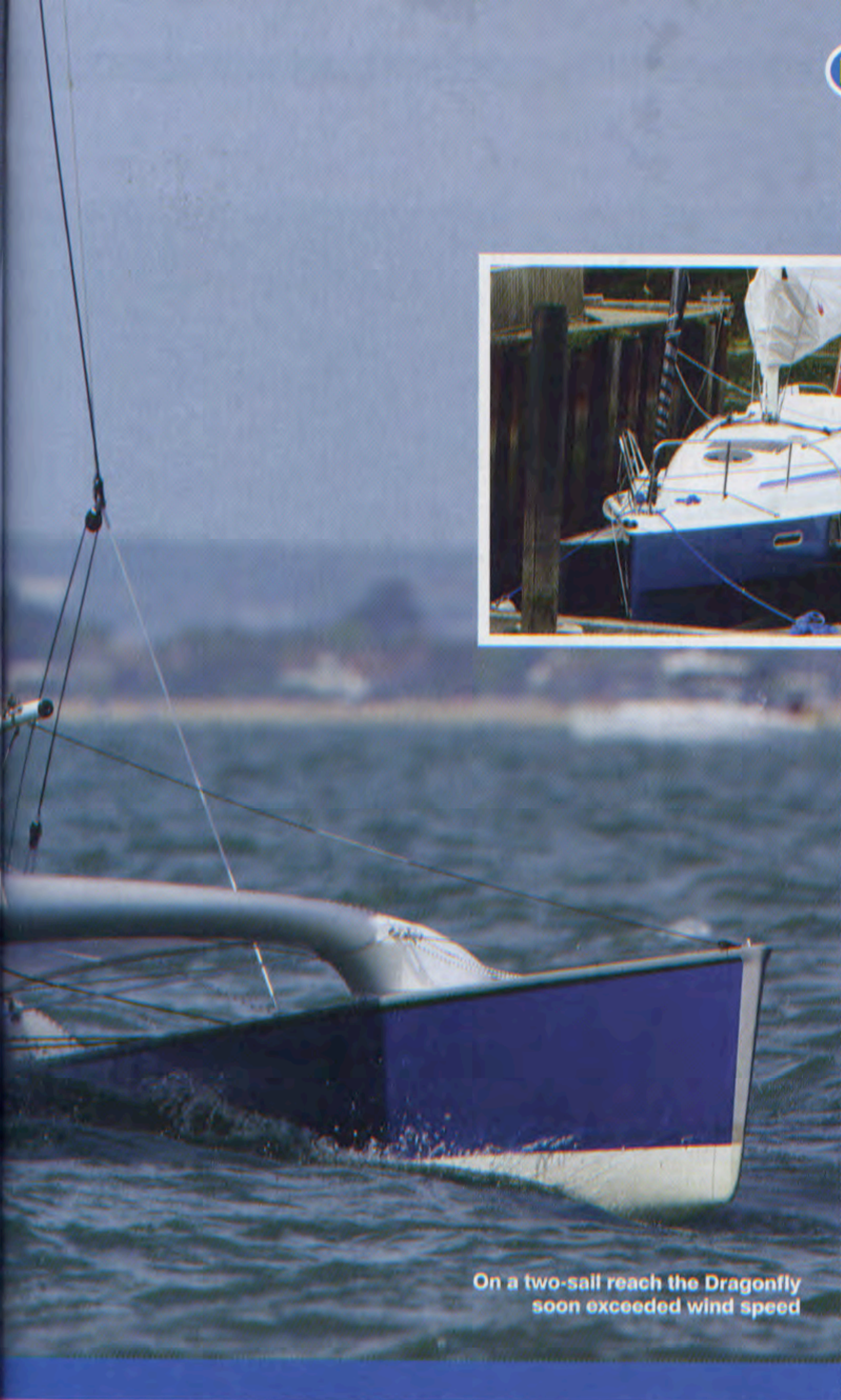
ABOVE High-performance beach-boat: the Dragonfly floats in next-to-nothing. INSET Wings folded: with the outriggers tucked beneath the main hull, the beam is reduced to just 2.55m (8ft 4in)
