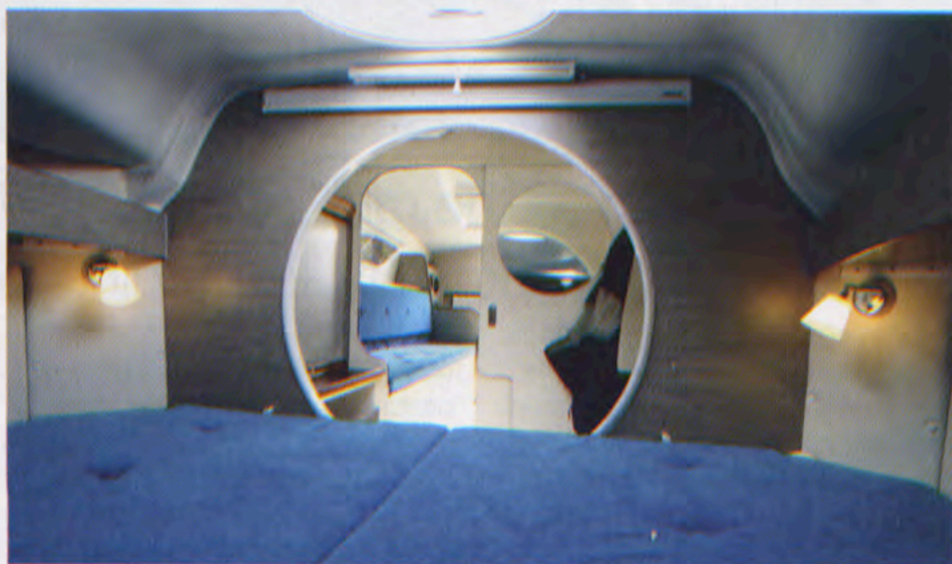
The massive forward bulkhead takes the load of the outriggers' beams and water-stays; hence the relatively small aperture to the forecabin
