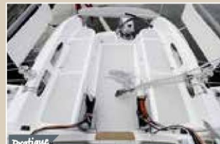
Pratique The rigging is brought back into the coaming, under the lifting seats.
