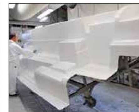
▲ The backing mould inside is very thin. Everything that can be in-built is; even the washbasin in the head, to reduce weight.
