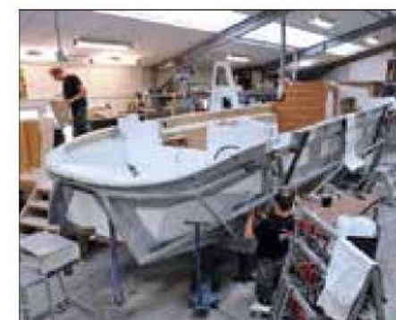
▲ The hulls are placed in casing to prevent any distortion while the structural parts and accommodation are installed.
