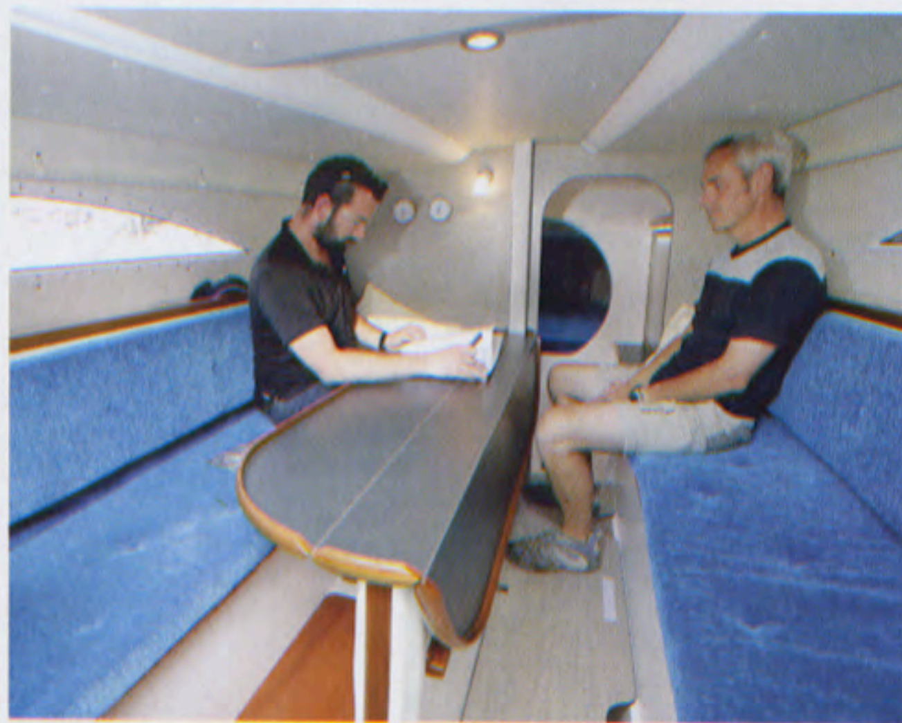
The coastal cruising saloon dines six but lacks ventilation. With the grey sole panel folded up, it's easy to walk forward
